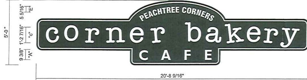
(A) S/F R.O.P.T. WALL MOUNTED (FLUSH) INTERNALLY ILLUM. SIGN SCALE: 3/8" = 1'-0" (1) ONE REQUIRED - MANUFACTURE & INSTALL
