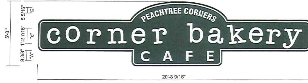
(A) S/F R.O.P.T. WALL MOUNTED (FLUSH) INTERNALLY ILLUM. SIGN SCALE: 3/8" = 1'-0" (1) ONE REQUIRED - MANUFACTURE & INSTALL
