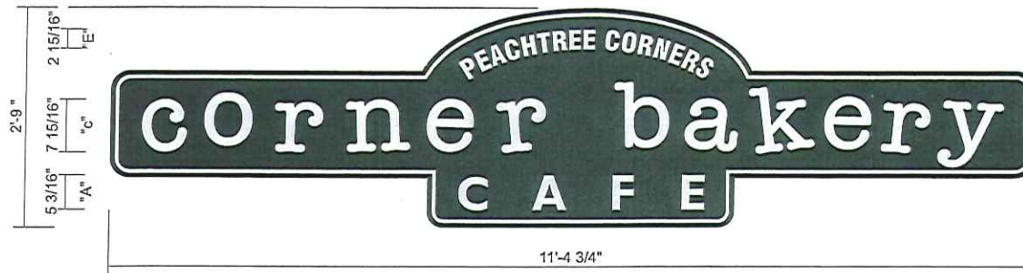
(H) S/F R.O.P.T. WALL MOUNTED (FLUSH) INTERNALLY ILLUM. SIGN SCALE: 3/4" = 1'-0" (1) ONE REQUIRED - MANUFACTURE & INSTALL
