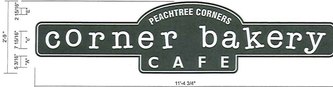
(H) S/F R.O.P.T. WALL MOUNTED (FLUSH) INTERNALLY ILLUM. SIGN SCALE: 3/4" = 1'-0" (1) ONE REQUIRED - MANUFACTURE & INSTALL
