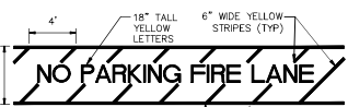
NOTE: VERGAGE "NO PARKING FIRE LANE" BETWEEN PARALLEL LINES EVERY 100' OR AT LEAST ONCE IN FIRE LANES SHORTER THAN 100'. FIRE LANE STRIPING NOT TO SCALE
