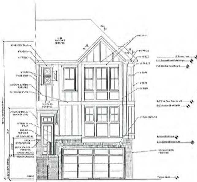
FRONT ELEVATION D - LOT 13 KITCHEN FRONT SCALE: 1/8\"/>
