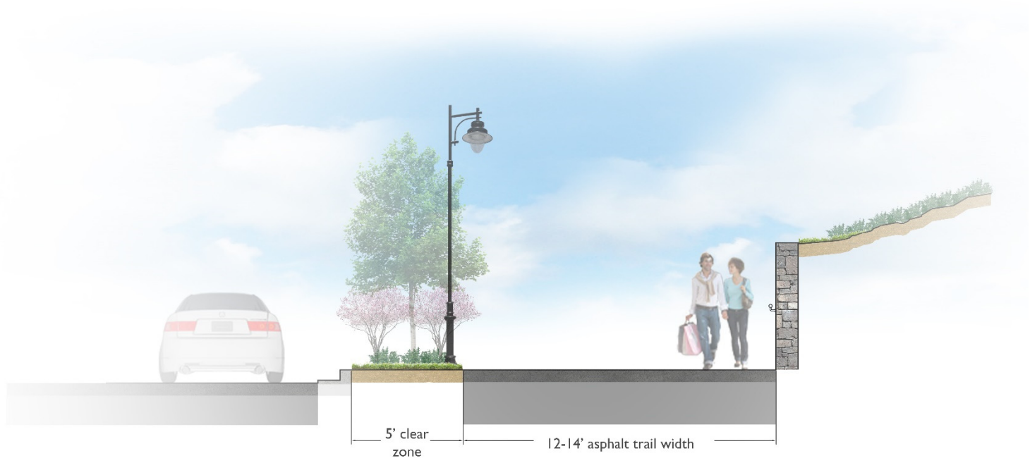
Figure 4.4 Typical cross section of side path with concrete wall and handrail
