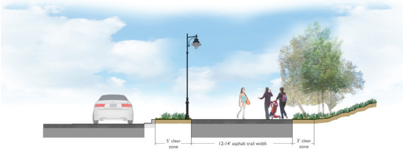
Figure 47. Typical cross-section of a side path trail, Gwinnett Countywide Trails Master Plan
