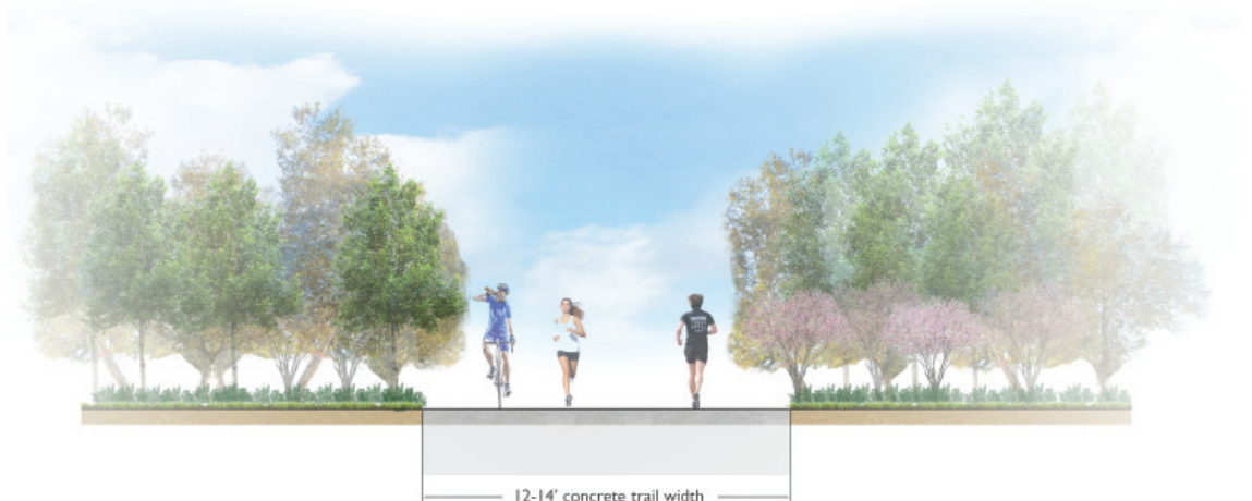
Figure 46. Typical cross-section of an off-road trail, Gwinnett Countywide Trails Master Plan
