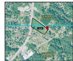
FLOOD MAP N.T.S. THIS PROPERTY IS NOT LOCATED IN A FLOOD HAZARD ZONE PER F.E.M.A. FLOOD INSURANCE RATE MAPS OF GWINNETT COUNTY, GEORGIA. COMMUNITY PANEL NO. 13135C 0151F & 13135C 0145F EFFECTIVE DATE SEPTEMBER 29, 2006.
