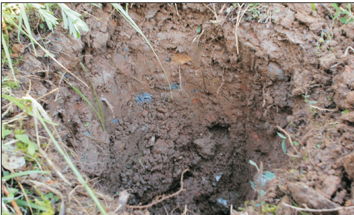
B. Disturbed soil profile associated with the sewer line construction.
