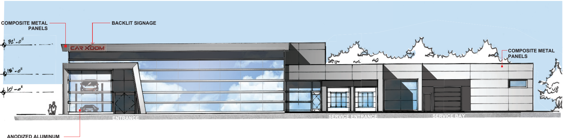
SIDE ELEVATION - MCDANIEL BRIDGE ROAD VIEW SCALE: 1/16" = 1'-0"
