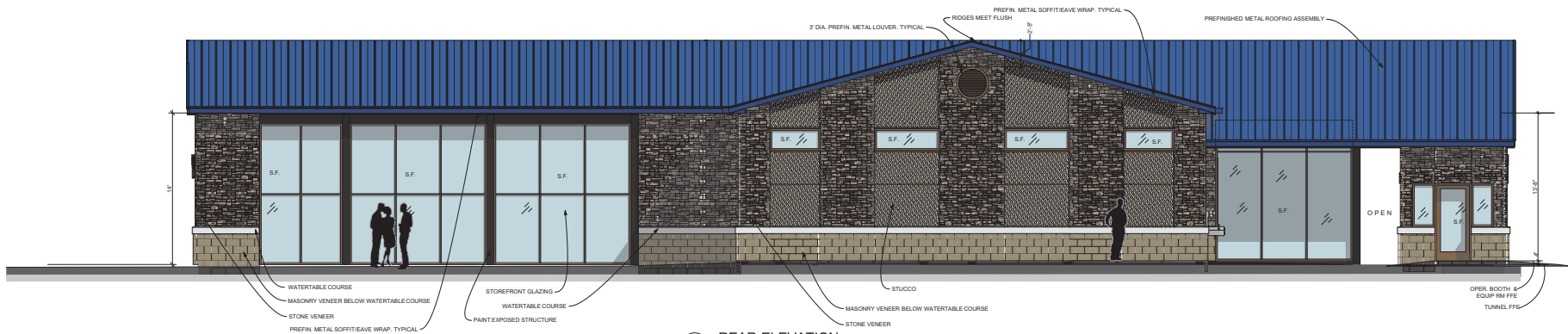
1 REAR ELEVATION SCALE 1/4" = 1'-0"
