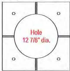
Top 20"x20"x1/2" Steel Plate for 12.75" Pipes Qty: 2 WaterJet
