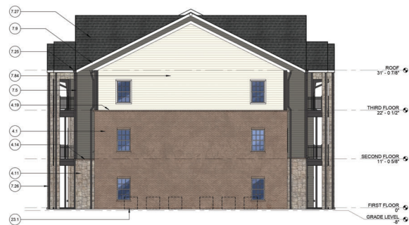
3 BUILDING FOUR RIGHT SIDE ELEVATION 1/8" = 1'-0" BRICK/STONE COVERAGE: 87.6%
