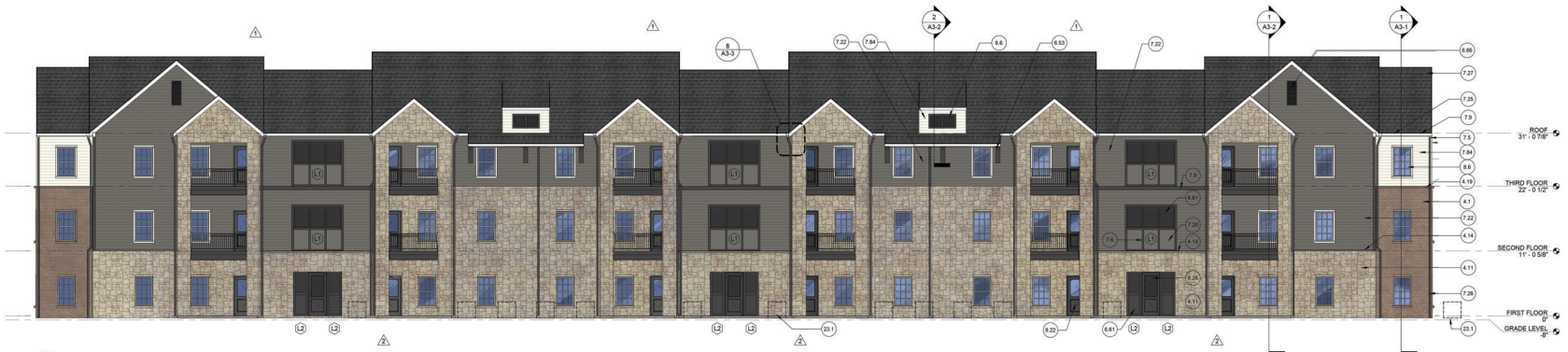
2 BUILDING FOUR REAR ELEVATION 1/8" = 1'-0" BRICK/STONE COVERAGE: 83.6%
