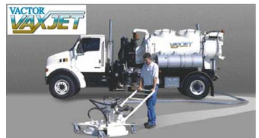
**Vacuum Closed Loop Discharge Systems:** These systems are capable of pressure washing and vacuuming up generated washwater simultaneously for disposal to an appropriate location. Once again these systems utilize a
