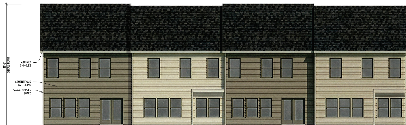
24' FRONT ENTRY REAR ELEVATION 1/4" = 1'-0"
