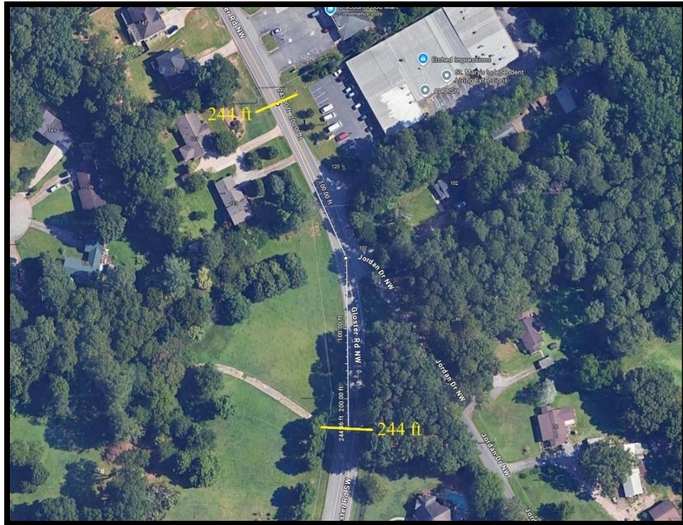
Figure 3 – Aerial Photograph of Gloster Road at Jordan Drive Showing Spacing Distances to North and South
