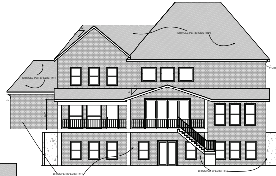
REAR ELEVATION West Facing 1/8"----1'-0"
