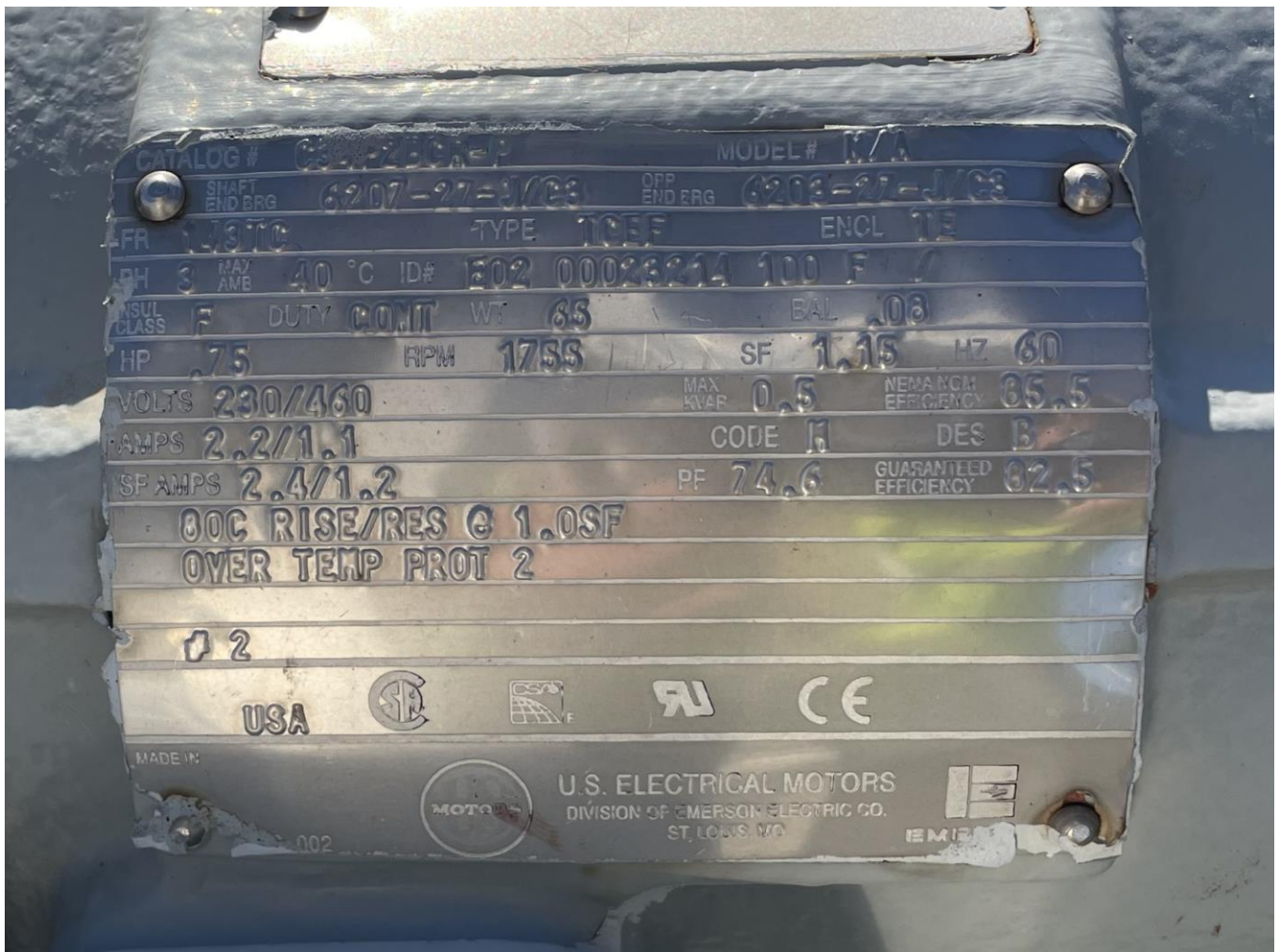
Photograph 8: Drive Unit Motor Name Plate
